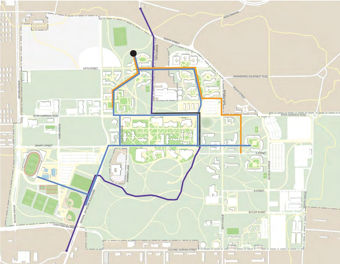
Stormwater runoff should be collected throughout the site and transported, mostly through surface conveyance, to LID water quality treatment areas. These areas will act to evapotranspire, infiltrate, or treat the water. Overflow volumes will be released to a campus-scale storm drain network that leads to larger percolation landscapes.
