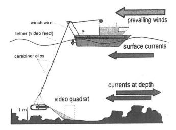
significantly, allowing for better positioning over these maps for subsequent data analyses. We suggest either using a beacon and tracking program software (e.g., Trackpoint II/III, Edge-Tech) or manually estimating the distance of the sled from the stern of the ship (e.g., angle measurement and Pythagorean calculation) for more accurate mapping of transects.
